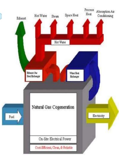
Cogeneration of Heat & Power- CHP is the simultaneous production of electricity and useful heat in one process.
